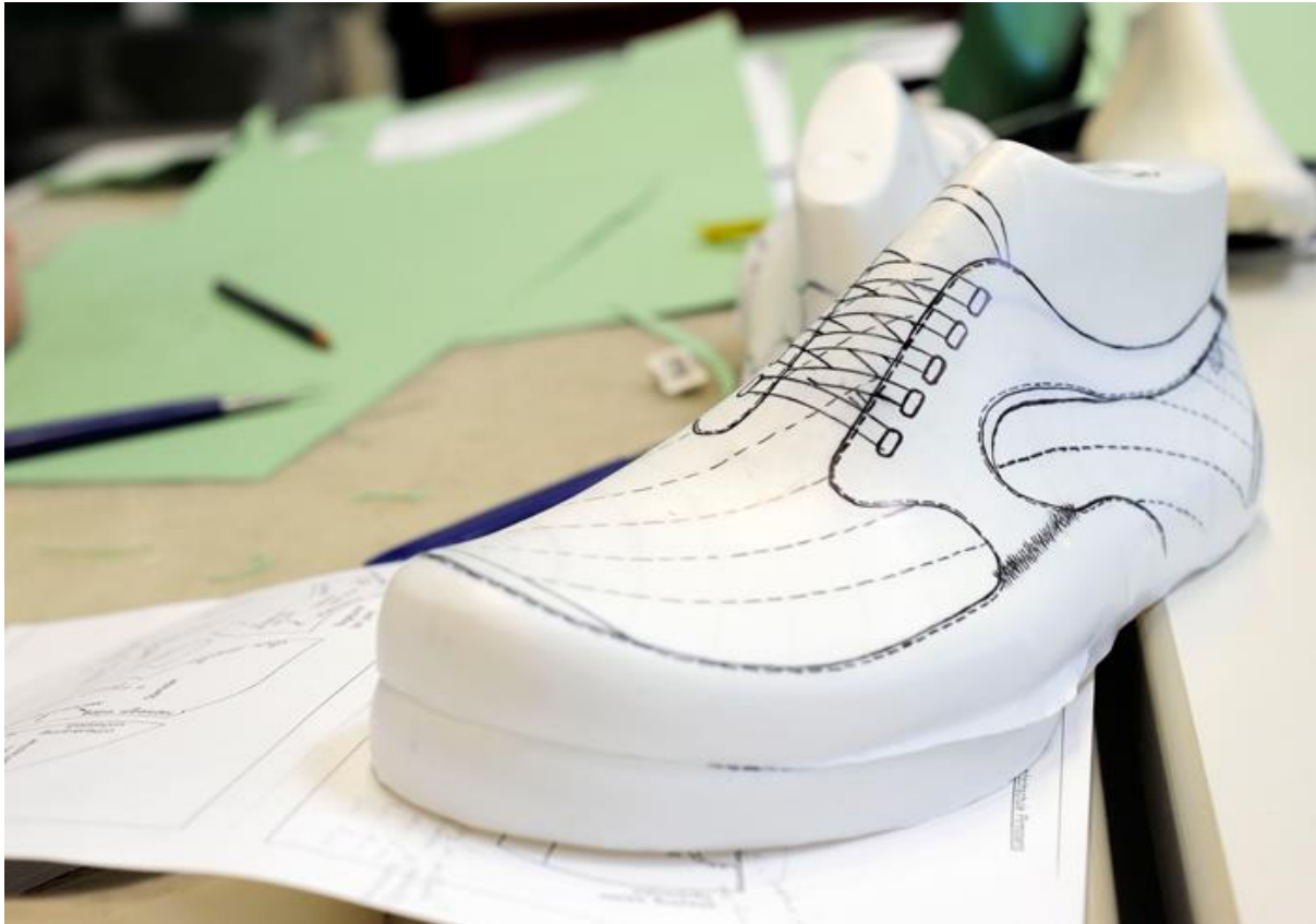
Fig. 3: Design sketch of a men's shoe on a deep draw copy (a plastic shell). Credit: ISC / Schuhkurier
