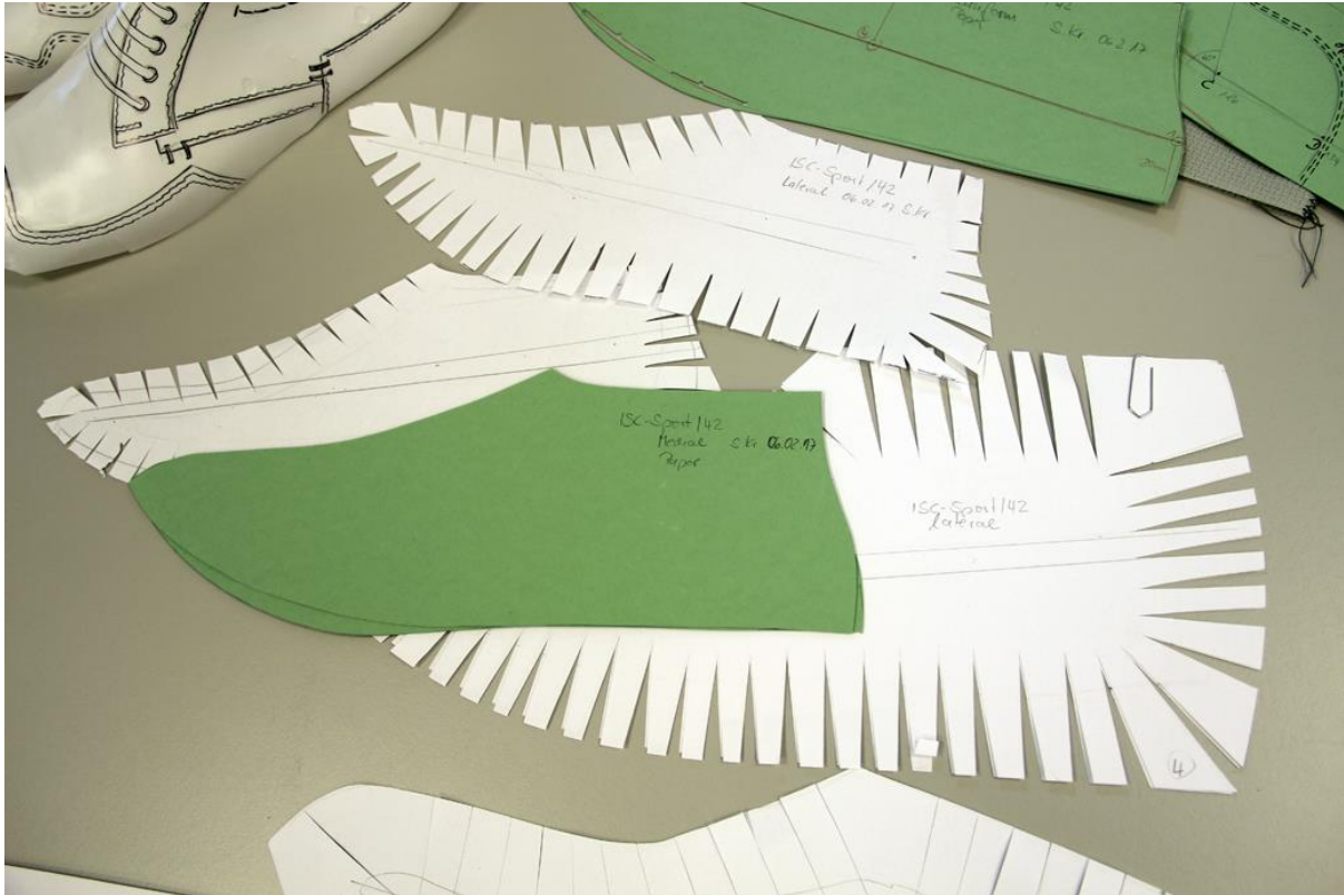
Fig. 5: Another method to flatten the last surface from 3D to 2D is producing a slotted form. Credit: ISC
