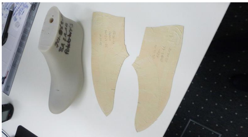
Fig. 6: The lateral and medial last copies are transferred onto cardboard. Credit: Gabor
