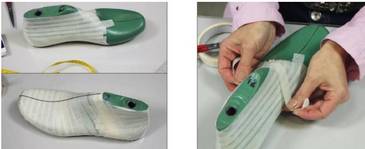
Fig. 4: Making a tape copy. Credit: ISC
