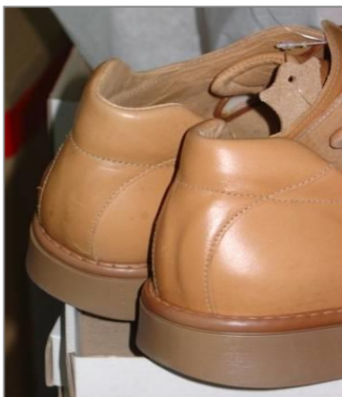
Fig. 17: Leather marks caused by backing materials
