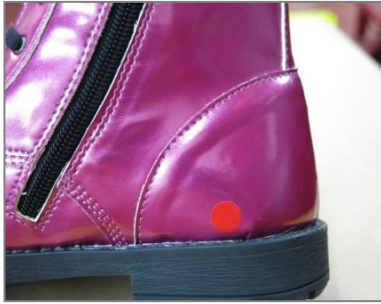
Fig. 18: Wrinkles caused by deficiencies in assembling operations
