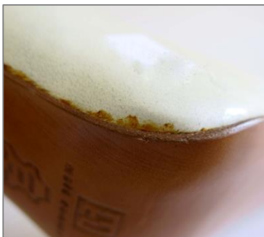
Fig. 16: Glue stains and visible stitch marking
