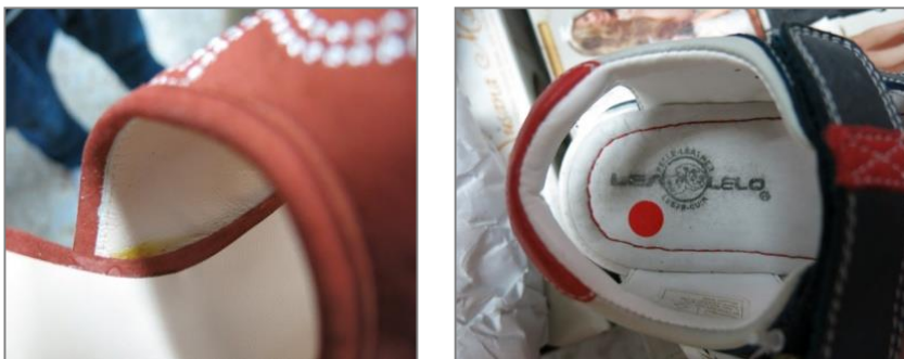
Fig. 25: Presence of stains, lining creases, right insock stamping
