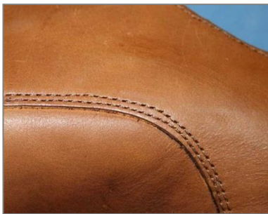
Fig. 19: Parallel seams, corrected stitches
