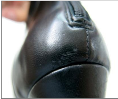
Fig. 14: Presence of wrinkles, scratches or imperfections on leather
