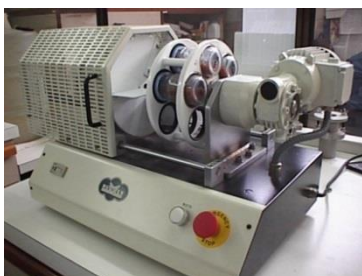
Fig. 38: Water vapour permeability
