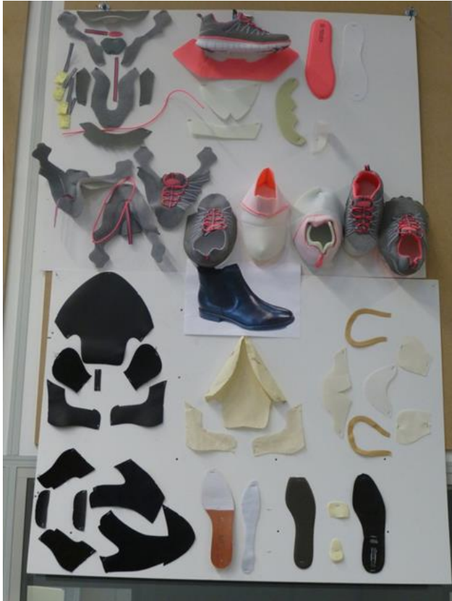
Fig. 1: Views of shoe parts like on this photo can be very helpful for the trainee to understand the complexity of a shoe
