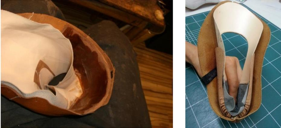
*Fig. 3: Aplicar el contrafuerte; Fuente: <http://denishoe.blogspot.com/2013/07/lasting-7-wrapping-last-with-upper.html>*
