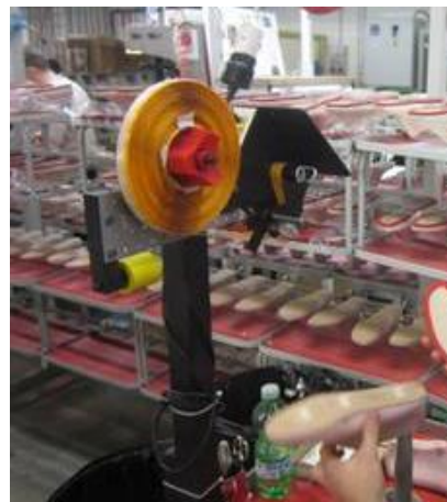
Fig. 9 Applying the insole to the last using tape; Source: www.tapepeel.com/en/tapepeel/
