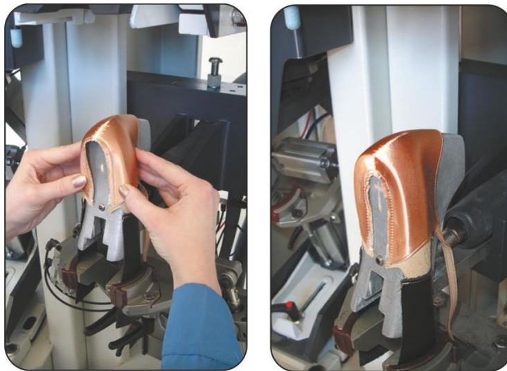
Fig. 4: Back-part pre-moulding, Source: https://www.olympicld.gr/en/multiform4
