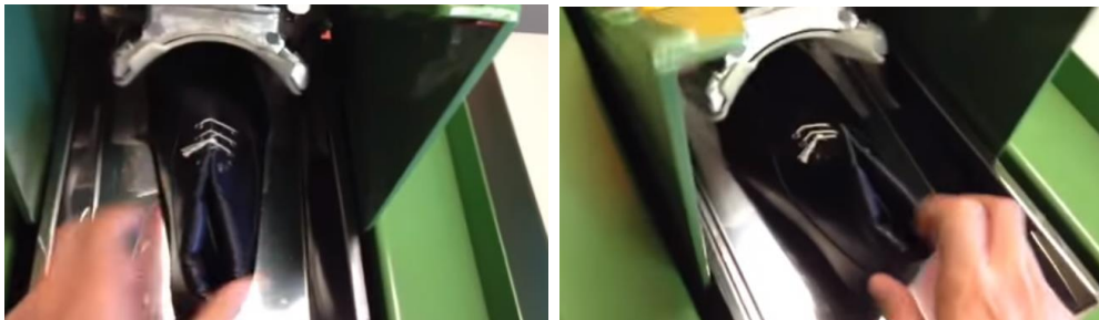
Fig. 7: Conditioning the uppers; Source: www.olympicltd.gr/gr/x-treme-soft-48-2
