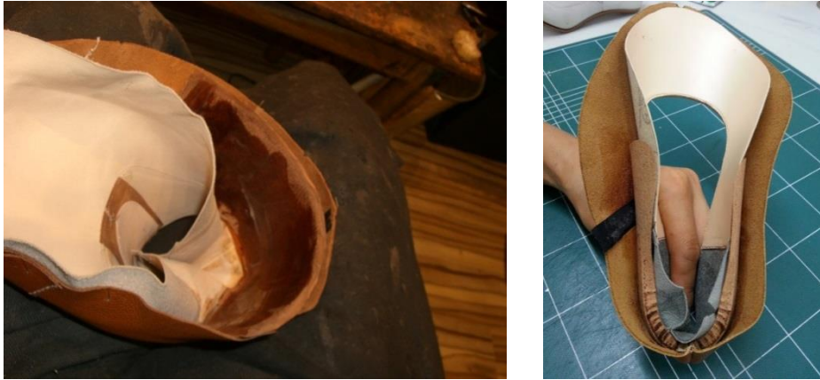
Fig. 3: Applying the stiffener; Source: http://denishoe.blogspot.com/2013/07/lasting-7-wrapping-last-with-upper.html
