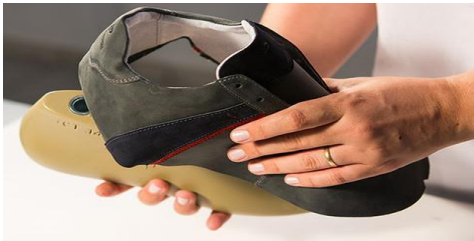
Fig. 39: Position the upper on the last
