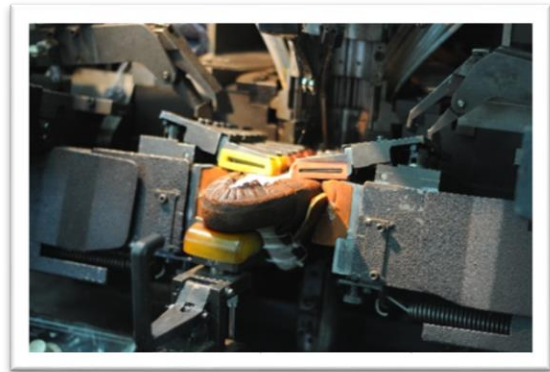
Work-based learning / Heat setting machine; Source: Carité
