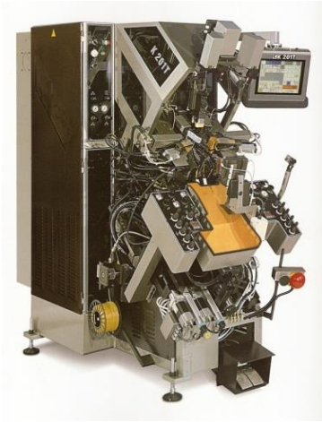
Fig. 38: Forepart lasting machine
