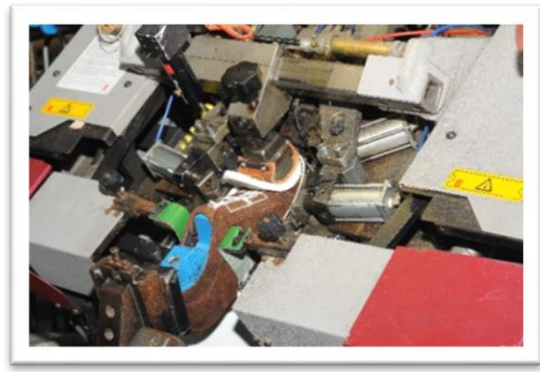
Work-based learning / Positioning upper on the last; Source: Carité
