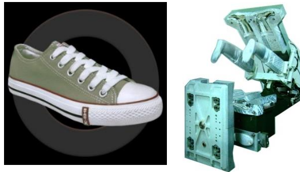
Fig. 24: Vulcanization lasting shoe
