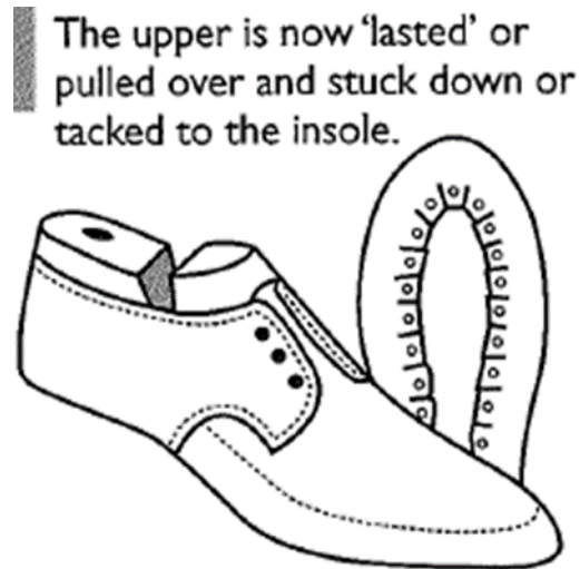
Fig. 2: The shoe lasting
