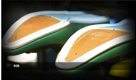
Fig. 21: Goodyear lasting shoe
