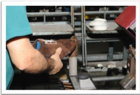
Work-based learning / Positioning upper on the last; Source: Carité
