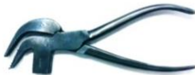
Fig. 43: Lasting pliers: tool to adjust the height of the shoe
