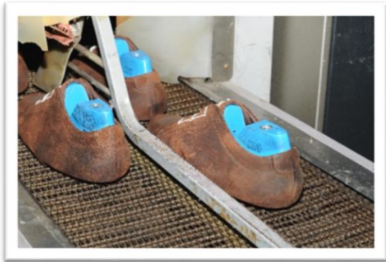
Work-based learning / Heat setting machine; Source: Carité
