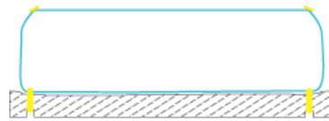
Fig. 16: Scheme of the mocassin lasting
