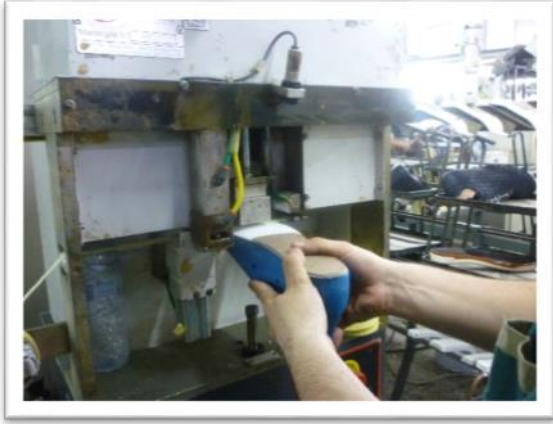
Work-based learning / Applying the insole on the last; Source: Carité
