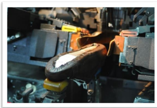
Work-based learning / Side and seat lasting; Source: Carité
