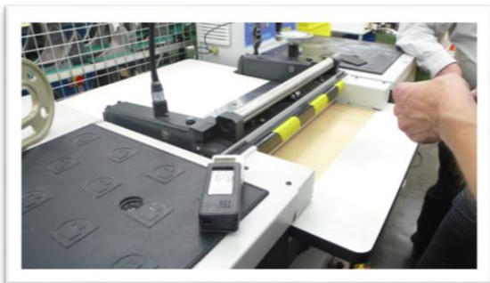
Fig. 34: The parts are split to attain homogenous thickness.
