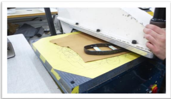
Fig. 37: The sock liners are cut with cutting dies on a swing-arm clicking press.
