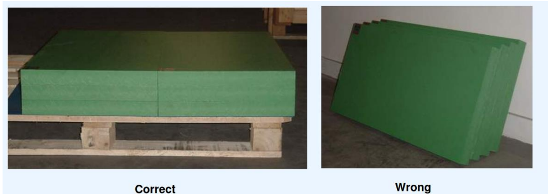
Fig. 24: Correct (horizontal) and wrong storage (vertical) of cutting boards
