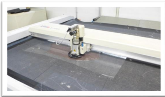
Fig. 32: The upper parts are being cut.
