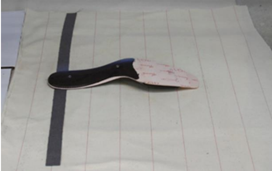
Fig. 15: Insole and piping strip to be glued around the edge. Credit: Gabor
