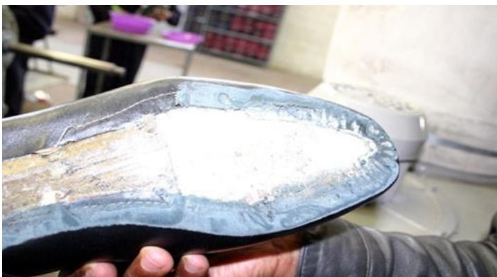
Fig. 6: Example of an over-roughed upper: the white interlining is showing through. The strength of the sole bond will now completely depend on the structural strength of lining and interlining. Credit: ISC
