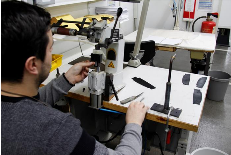
Fig. 13: Clamping device used for covering heels with leather. Credit: Gabor
