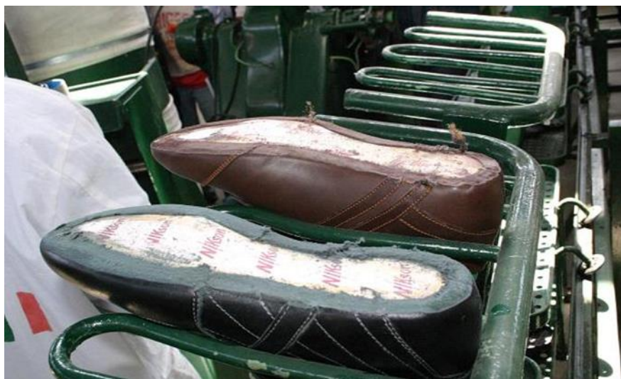
Fig. 7: If roughing dust remains on the roughed surface, it will be covered with glue in the next step, which will ultimately weaken the bonding strength. Credit: ISC
