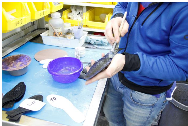
Fig. 11: Cement is applied to the sole. Credit: Gabor
