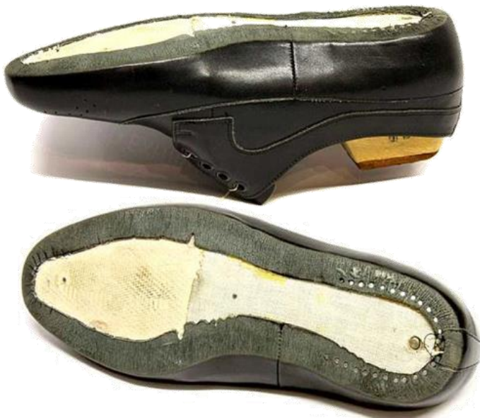
Fig. 5: Perfect roughing result: Only the grain layer has been removed. The structural strength of the upper leather is maintained and the contact area for the adhesive bond has been enlarged. Credit: ISC
