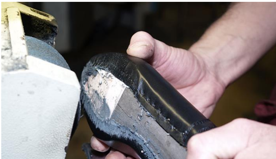
Fig. 3: Manual roughing (coarse sand paper). Credit: ISC
