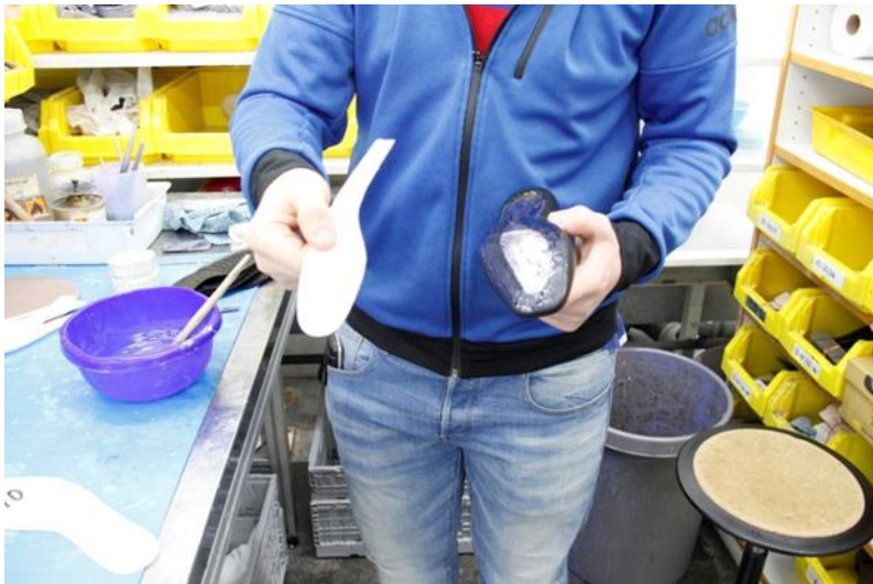
Fig. 10: The bottom filler's function is to level out the difference in height between the lasting edge and the insole. Credit: Gabor
