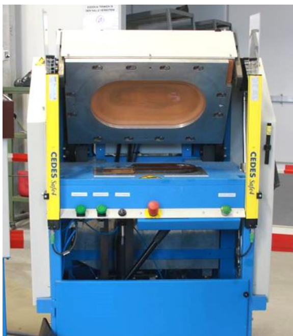
Fig. 19: Double membrane pneumatic sole press. Credit: ISC
