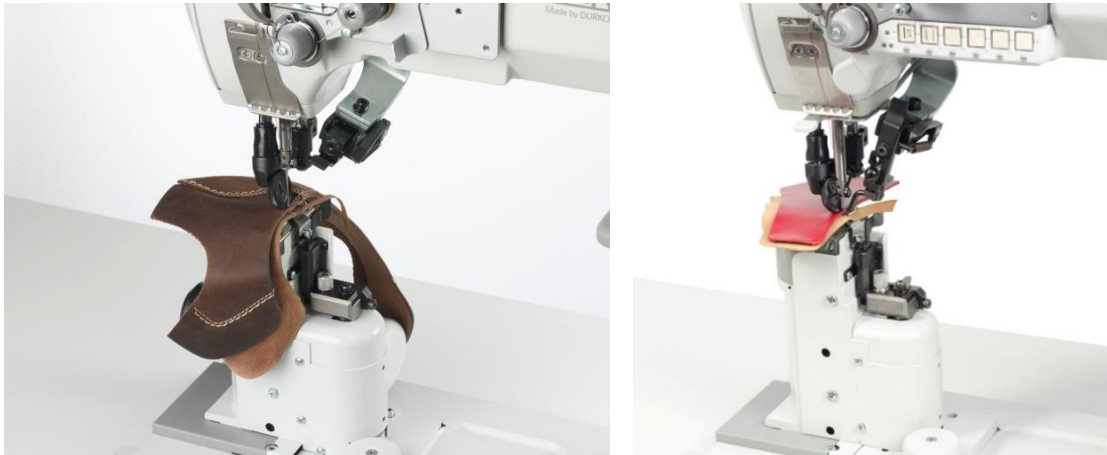
Fig. 3: Post bed machines with integrated direct drive for inserting lining and undertrimming; Source: www.minerva-boskovice.com/888-356020
