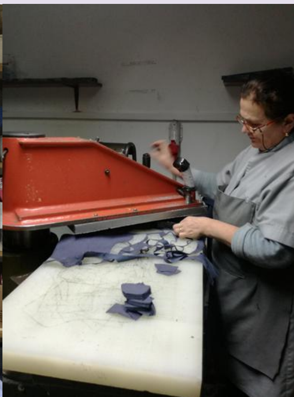
Fig. 3 Cutting operation using press machine
