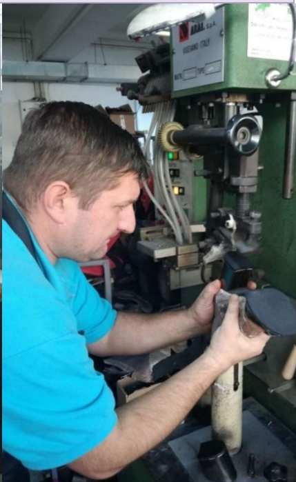
Fig. 29 Machine for heel attachment
