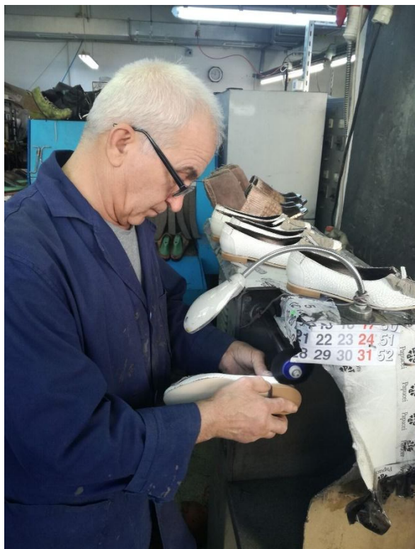
Fig.29 Heel paring/ sole edge paring
