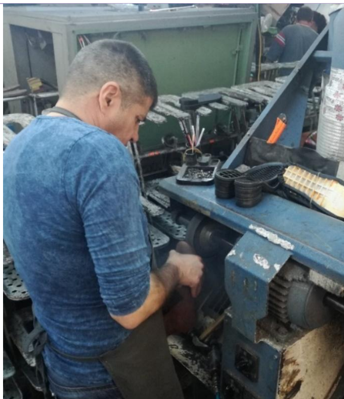
Fig. 24 Bottom roughing (lasting allowance and sole)
