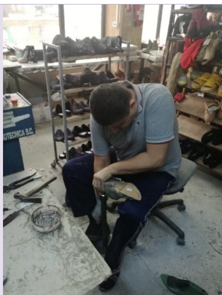
Fig. 19 Positioning the uppers on the last
