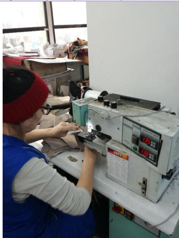
Fig. 8 Edge folding operation
