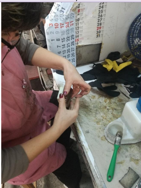
Fig. 24 Bottom roughing (lasting allowance and sole)
