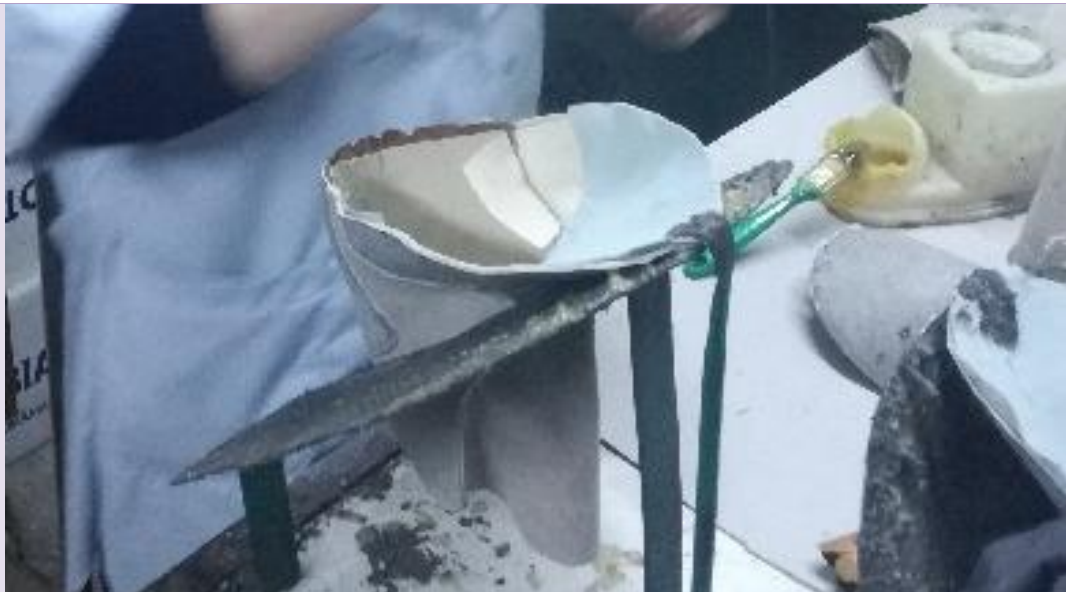
Fig. 16 Applying toe puff using hot press
