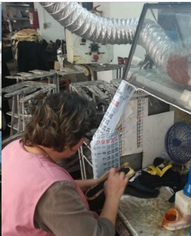
Fig. 25 Applying the adhesive on the sole and allowance
